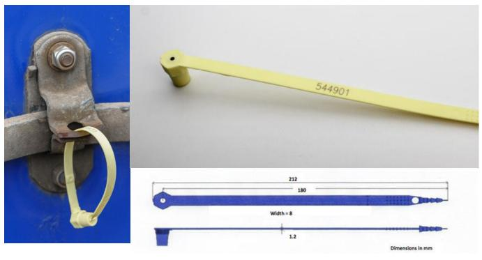
The Talisman Ringloc seal is a fixed length seal manufactured from polypropylene, with a polyacetal locking jaw with a double locking action which provides a positive locking action.
