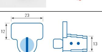
The Talisman Meterloc is a very flexible security seal, comprising a two piece plastic body and a wire, which can be supplied with a variable length to suit customer requirements.
