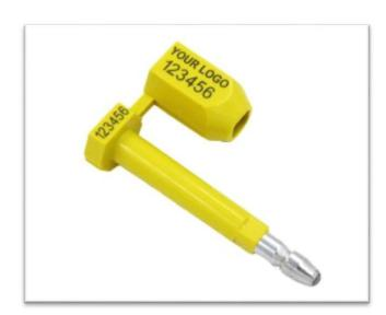
The Talisman Cargoloc is a heavy duty barrier seal comprising of a metal pin which has a 45mm sealing length and 22.5mm long barrel, total length of sealed unit is 94mm long, all of which is coated in high visibility plastic.
